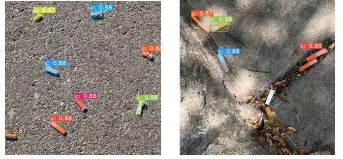
Fig. 3. Sample results are shown on two images from the Cigarettes dataset in the form of confidence scores, segmentation masks (overlayed over each instance) and bounding boxes (around each instance).
